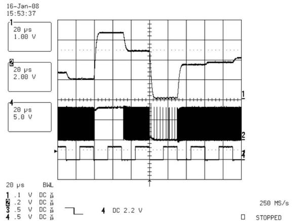
Fig. 8. Waveforms from the chaotic map/ $\Delta\Sigma$  block. From bottom to top: clock of the chaotic map; driving signal  $\xi(t)$  modulated by the  $\Delta\Sigma$  converter; and the same signal demodulated by an external low-pass filter.
