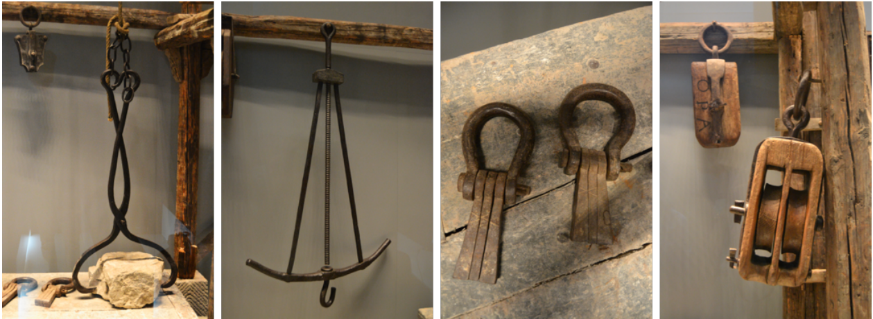
Fig. 1. Historical tools displayed in the Museo dell'Opera del Duomo. From the left: pincers, turnbuckles, three-legged lewis, pulleys.
