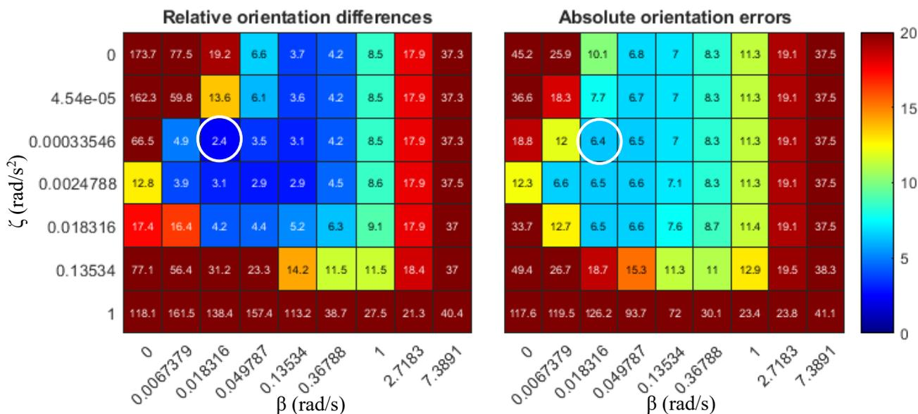
Figure 2: heatmaps of the relative orientation differences vs absolute orientation errors averaged over the two MIMUs for MAD (fast rate). In this case the two selected values of  $\beta$  and  $\zeta$  minimized both the relative differences and the absolute errors. All the units are in degrees.
