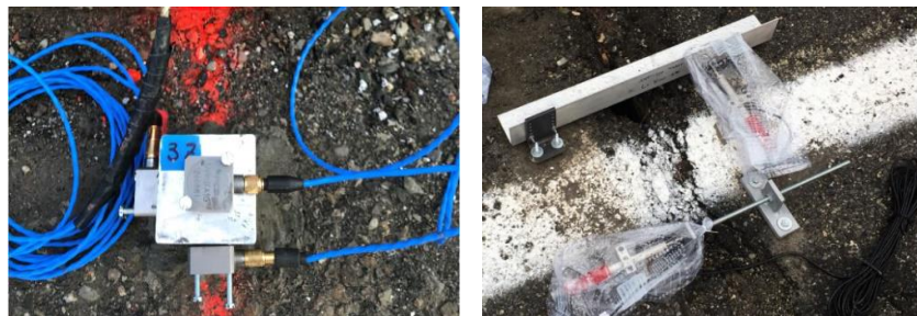
Fig. 2. mono-axial accelerometer PCB (a); LVDT (b).
