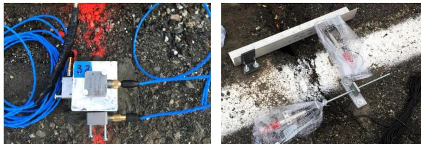
**Fig. 2.** mono-axial accelerometer PCB (a); LVDT (b).
