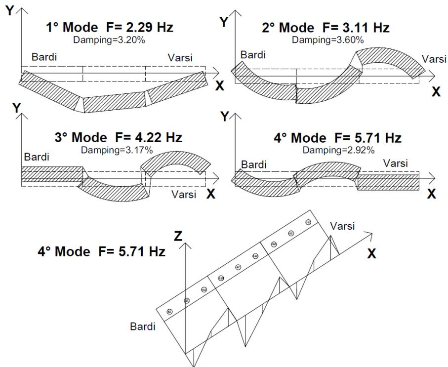
Fig. 8. Schematic representation of the first 4 modal shapes.
