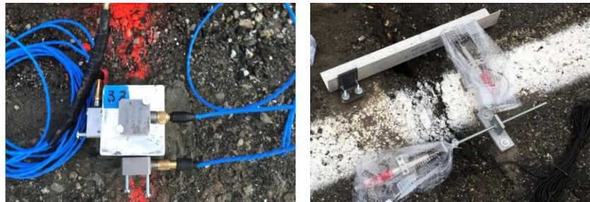
Fig. 2. mono-axial accelerometer PCB (a); LVDT (b).
