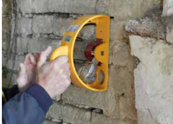
Figure 9. On site rebound test (credits Manuela Mattone)
