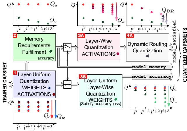
Fig. 8: Flow of Our Framework for Quantizing CapsNets.
