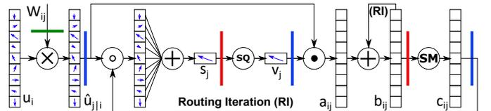
Fig. 9: Quantization of a capsule layer with dynamic routing. Colored bars show the arrays that are rounded and quantized. In green, the weights are quantized with  $Q_w$  bits. In blue, the activations are quantized with  $Q_a$  bits. In red, data are quantized more aggressively with  $Q_{DR}$  bits. The precision is lowered before complex and compute-intensive functions (*squash*, *softmax*).
