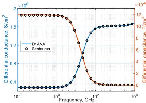
Fig. 2: Comparison of differential conductance and capacitance spectra of a *pin* diode (300 nm *p*-type  $10^{19} \text{ cm}^{-3}$  doped; 10 nm intrinsic layer; 300 nm *n*-type  $10^{19} \text{ cm}^{-3}$  doped), computed by D1ANA and Sentaurus Device.
