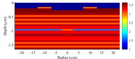
Fig. 1: Refractive index transverse section of the optical structure in a compact form (DBR multiplicity skipped) of investigated VCSEL [7]. Blue region ( $n = 1$ ) indicates air; the two relieves at the top are the metal contact placed above the a  $p^{++}$ -doped GaAs layer; the region between two light blue stripes is the oxide aperture. Below the QW region. The 110nm thick substrate is not shown.
