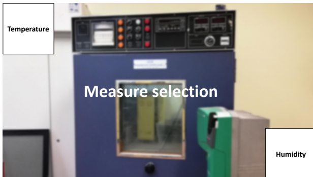
Figure 6: Example of an inspection task: measure selection menu, with flickering white squares for options (as usual in AR glasses, background image is blurred to focus on the selection).
