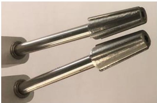
Figure 2. Two counter-rotating rasp cutting heads extract sample from the surface and throw the material up between them.
