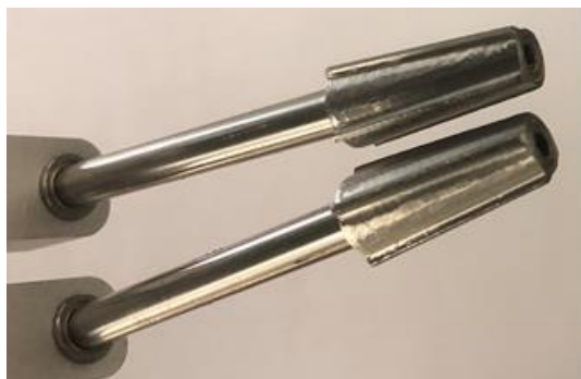
Figure 2. Two counter-rotating rasp cutting heads extract sample from the surface and throw the material up between them.
