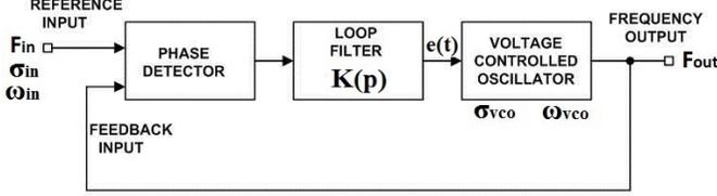
Fig. 1. The minimal structure of a PLL circuit
