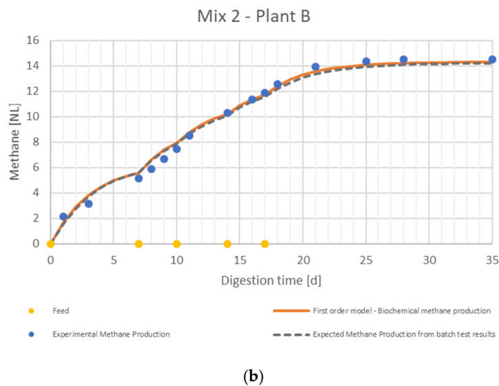
Figure 2. AD fed-batch tests. Measured points, simulated biochemical methane production curves, and expected biochemical methane production curves (validation of batch test results). (a) mix 1; (b) mix 2.
