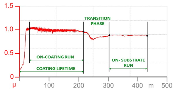
Fig. 7. Wear process stages with representation of the relevant portions of the friction curve
