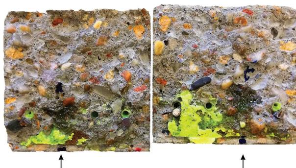
**Figure 11.** Crack surfaces (60 x 60 mm<sup>2</sup>) of one of the best performing CAPS specimen of lab 1. The hardened PU can be seen as fluorescent yellow. Arrows indicate the capsule from which fresh PU (visible as a dark stain) leaked on the surface when the specimen was broken. Image is highly saturated to improve visibility.
