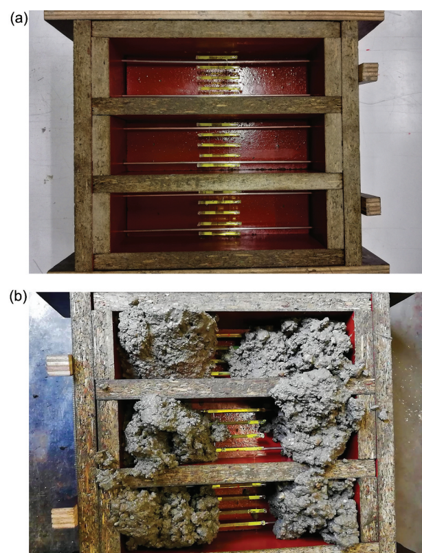
Figure 2. Moulds to make concrete specimens ( 60 \times 60 \times 220 \text{ mm}^3 ) with capsules (a: mould with five capsules; b: casting of specimens with four capsules).
