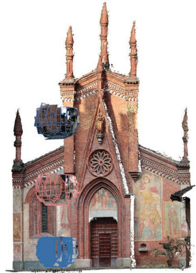
Figure 2. Different view of the position of the three automatic 360° acquisitions. Highlighted is the one used in the dataset B.
