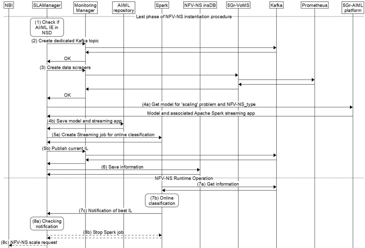
Fig. 2: 5Growth workflow to configure AI/ML-based scaling operation
