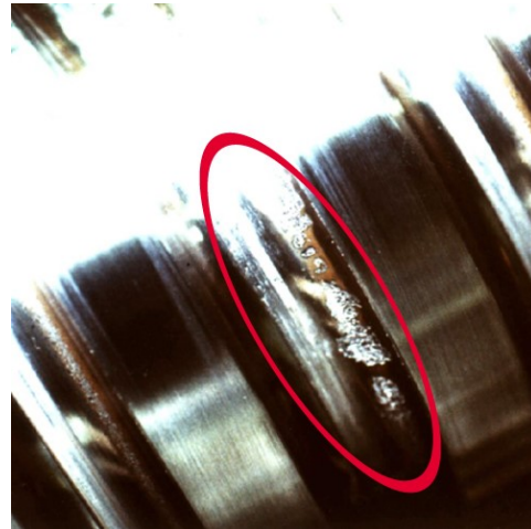
(d) Flaking/spalling of the screw raceway.
