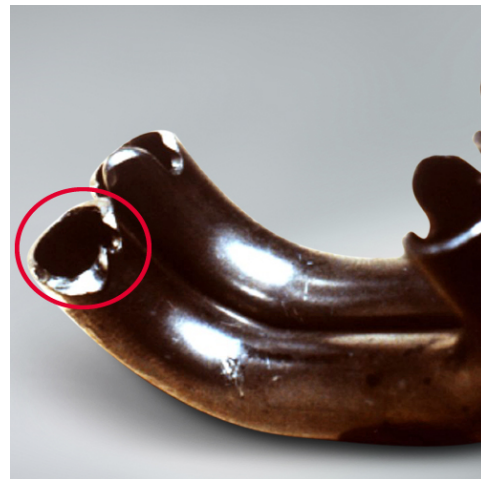
(f) Breakage of ball recirculation parts.
