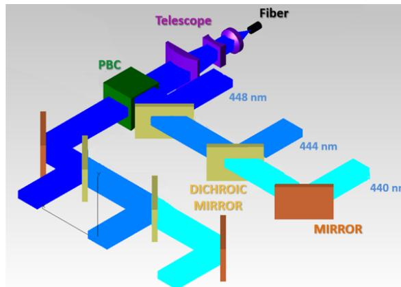
Figure 2. Scheme of the module optical architecture.
