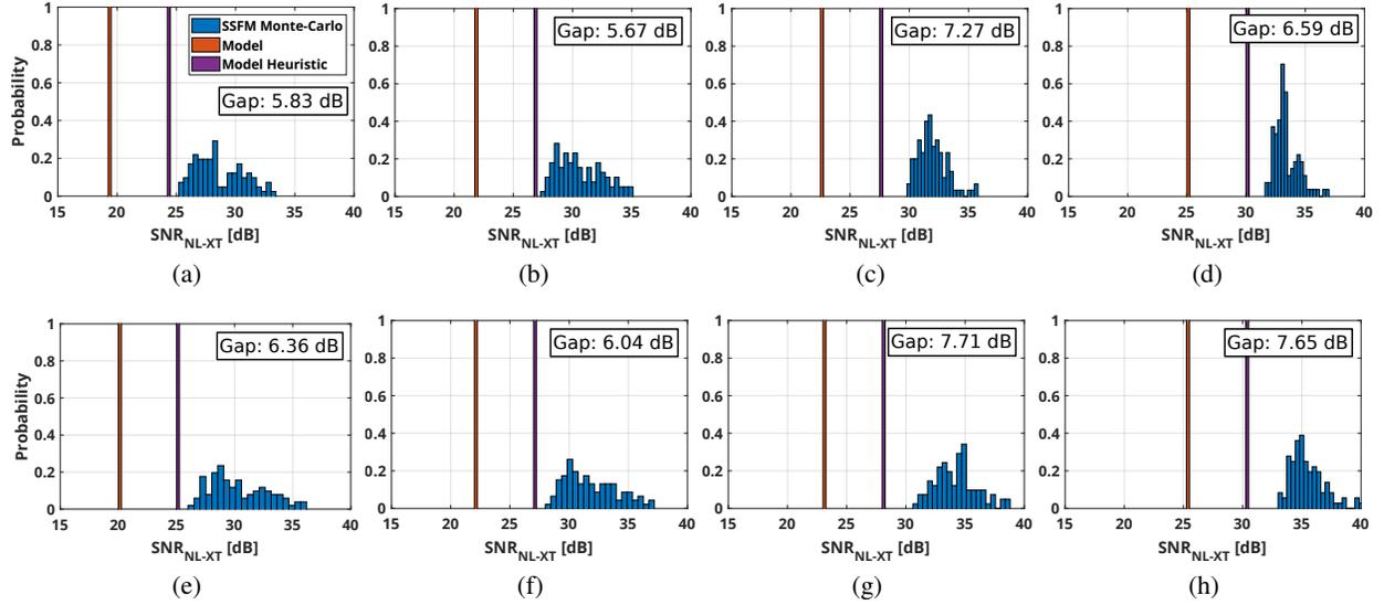
Fig. 3: Model vs SSFM pump and probe Monte-Carlo simulations:  $D = 4$  (upper row), 12 ps/(nm · km) (lower row).  $D_{RES} = 50$  (a,b,e,f), 90 ps/(nm · km) (c,d,g,h). Frequency spacing: 100 GHz (a,c,e,g), 200 GHz (b,d,f,h)
