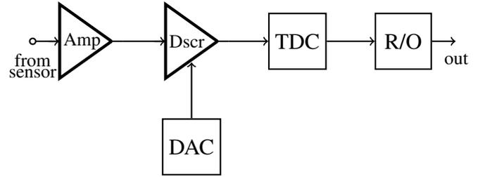
Fig. 1. Block diagram of the pixel read-out circuit.
