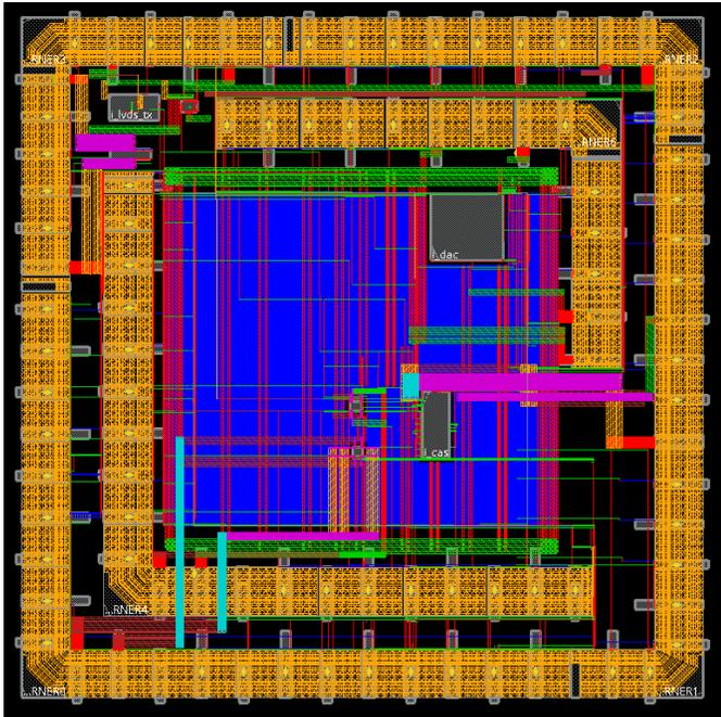
Fig. 4. Layout of the first chip prototype.
