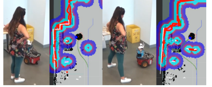
Fig. 1. The Sen3Bot human obstacle avoidance behaviour.
