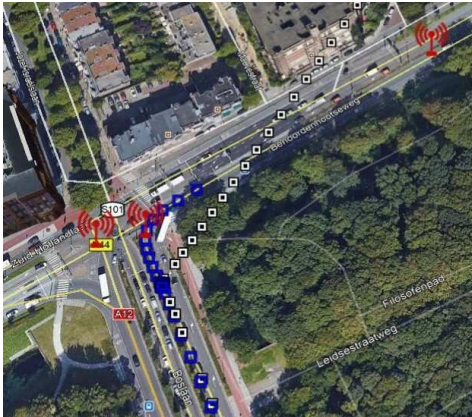
Fig. 4. Biased navigation solution due to the interference and multipath effect.
