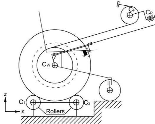
**Fig. 8.** Functional design of the wheelchair trainer
