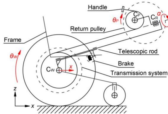
**Fig. 1.** Functional design of Handwheelchair.q
