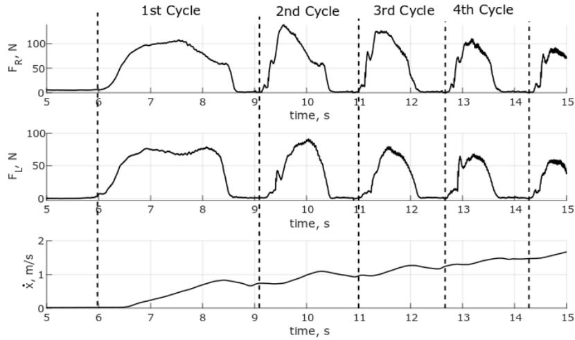
**Fig. 6.** User force and wheelchair speed during the acceleration phase
