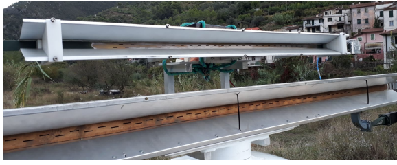
Fig. 6. TX (bottom) and RX (top) vertically polarized antennas used in P1b and P2a prototypes. Both launchers are slotted waveguides equipped with metallic flanges to shape the radiated field on the vertical plane.
