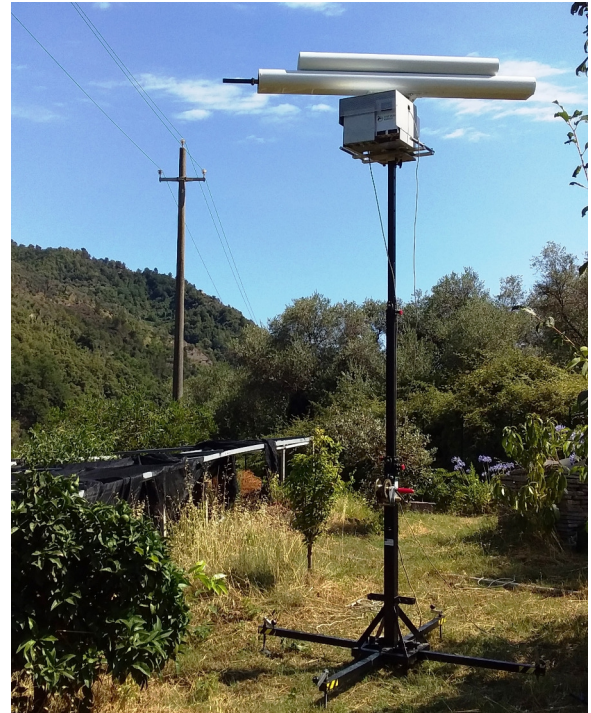
Fig. 1. Standard radar setup (P2b). The TX and RX antennas can be spotted on top of the system, covered by a radome. Most of the radar hardware was stored in the rack hanging right below the rotary joint. A telescopic tower helped to operate the radar up to about 6 m from the soil in order to avoid obstacles, such as trees or bushes.
