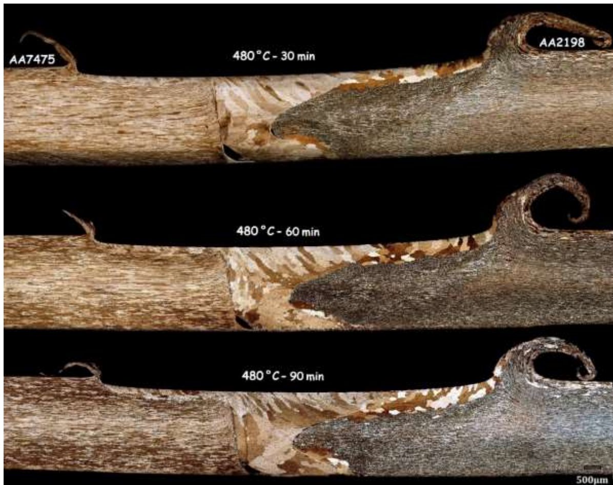
Fig. 12: Solution treatment of dissimilar joint of AA7475-AA2198 at 480 °C for 30 to 90 min.
