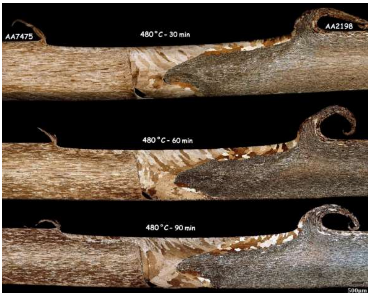
Fig. 12: Solution treatment of dissimilar joint of AA7475-AA2198 at 480 °C for 30 to 90 min. As illustrated, during annealing at 480 °C recrystallization of the new grains began from the weld surface. In the following, grains were elongated toward the bottom of SZ, and grain growth was
