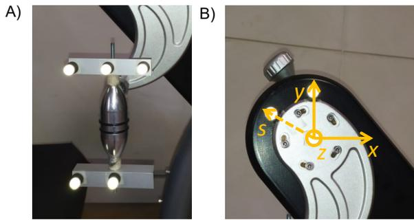
Fig. 2. A) Configuration of five markers on the right crank handle. B) GCS formed with three fixed markers on the support of the right crank arm.
