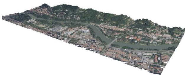
Figure 1. A view of the textured mesh of current state of the Valentino Park and its surroundings obtained with the aerial photogrammetric acquisition
