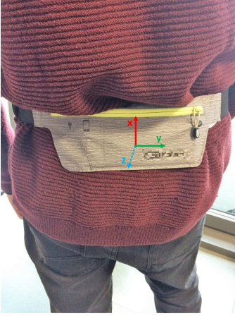
Fig. 1: Smartphone belt, smartphone position and reference axes
