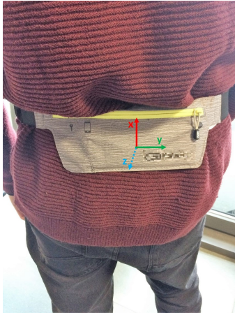
Fig. 1: Smartphone belt, smartphone position and reference axes
