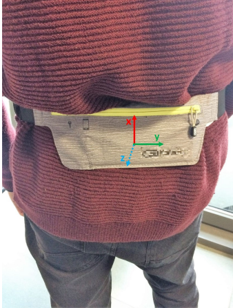
Fig. 1: Smartphone belt, smartphone position and reference axes
