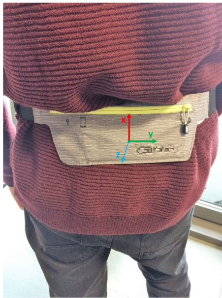
Fig. 1. Smartphone position adopted for the experiments.
