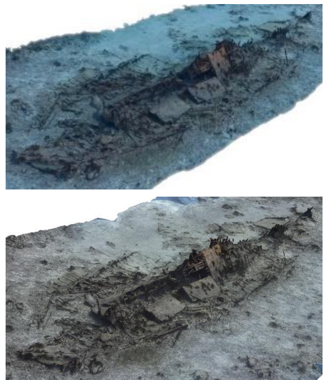
Figure 13. 3D model (triangulated mesh) of the Mandalay textured without using white balancing (top) and after the radiometric correction (bottom).
