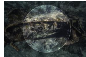
Figure 10. Circular mask adopted; the darker area will not be used during the calibration of the sensor and the feature detection (key-points) and matching (tie-points) steps.
