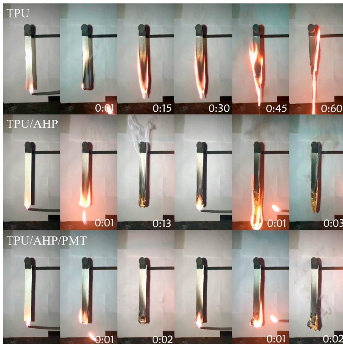
Figure 3. Video screenshots of TPU (thermoplastic polyurethane), TPU/AHP (thermoplastic polyurethane containing 10 wt. % of aluminum hypophosphite) and TPU/AHP/PMT (thermoplastic polyurethane containing 9 wt. % of aluminum hypophosphite and 1 wt. % of exfoliated montmorillonite decorated with phosphorylated chitosan) composites during UL-94 testing. Reprinted with permission from [30]. Copyright 2019, Elsevier.
