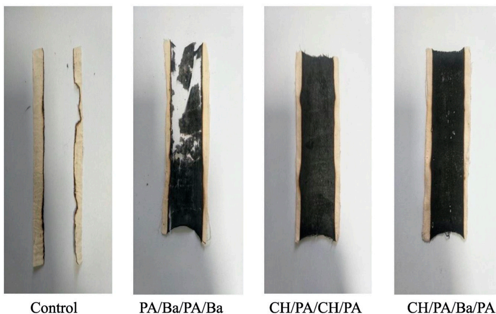
Figure 12. Residues at the end of the flame spread tests performed in a horizontal configuration. PA/Ba/PA/Ba: quad-layer made of phytic acid/ \text{Ba}^{2+} /phytic acid/ \text{Ba}^{2+} ; CH/PA/CH/PA: quad-layer made of chitosan/phytic acid/chitosan/phytic acid; CH/PA/Ba/PA: quad-layer made of chitosan/phytic acid/ \text{Ba}^{2+} /phytic acid. Reprinted with permission from [42]. Copyright 2019, Elsevier.
