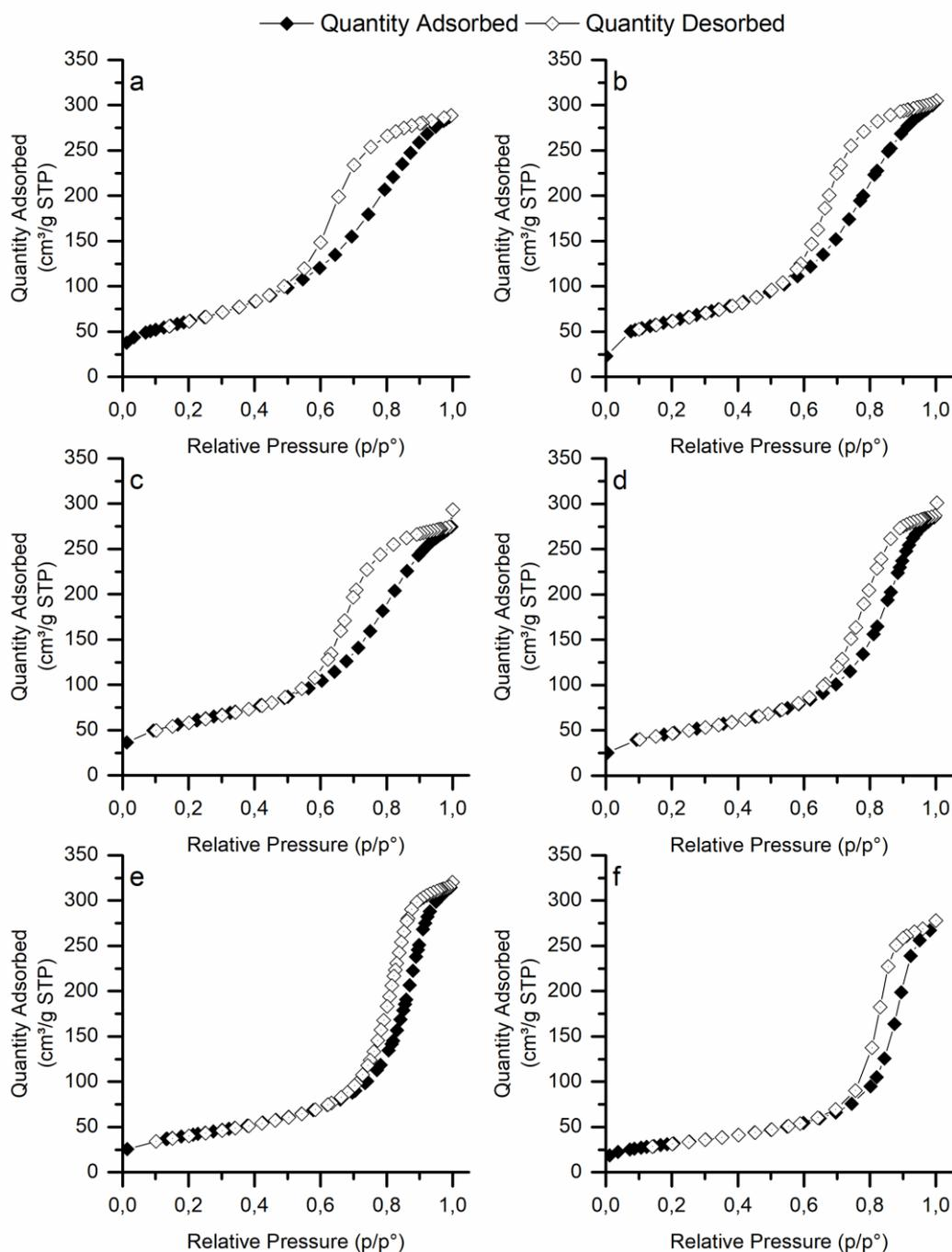
**Figure S-1:** Nitrogen adsorption isotherms for the a) fresh sample, b) fresh reduced, c) aged @ 270°C, d) aged @ 380°C, e) aged @ 425°C and f) aged @ 500°C
