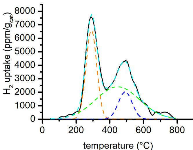
**Figure S-3:** H<sub>2</sub>-TPR with peak deconvolution
