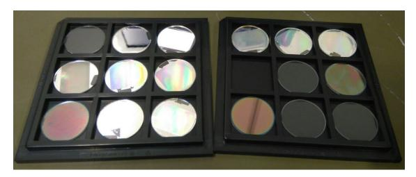
Figure 3.1: The reference and processed glass samples are shown after completing the NIL process for patterning of the diffraction gratings and deposition of the back reflectors.
