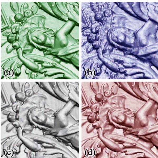
Figure 4. Particular of the meshes of the vault generated from the four datasets. (a) Faro Focus3D X 330, (b) Leica BLK360, (c) Leica RTC360, (d) Riegl VZ-400i.
