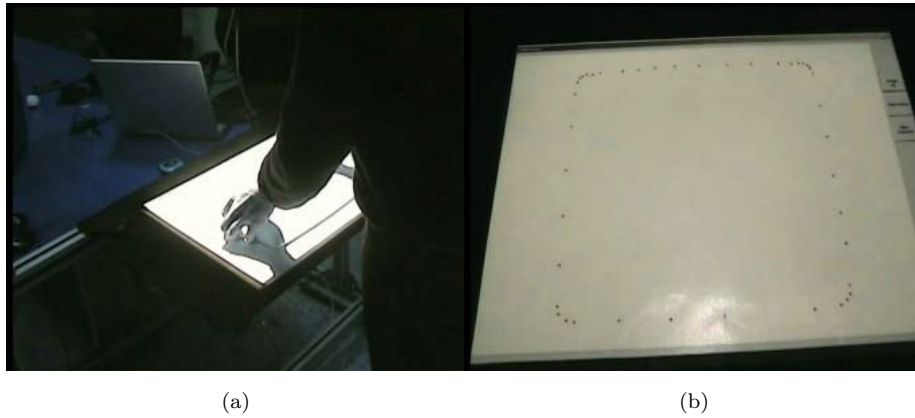
Figure 7: (a): a human operator is defining a projected AR path. (b): the result of the AR path generation. Images published in [57], licensed under CC BY 4.0
