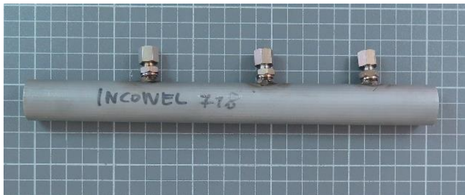
Figure 1 – (a) Drawing of the helically ribbed tube. All the quotes are expressed in [mm]. (b) Picture of one of the Inconel® tubes before the test campaign with the supports for the thermocouples (the squares in the background have 1 cm side).
