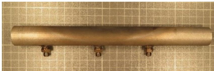
Figure 9 – (a) Emissivity vs sample temperature for Inconel® 718 in "as-received" condition [36], together with the trend line in Eq.16; (b) An oxidized sample tube after the test.
