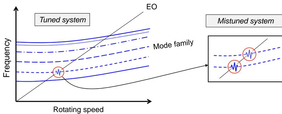
Figure 4. Splitting frequency in a mistuned system.
