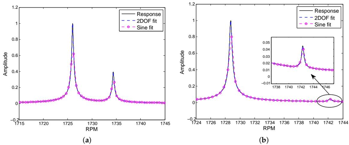
**Figure 9.** Comparison of non-dimensional amplitudes obtained by different fitting methods for  $EO = 7$  and  $\zeta_{1,2} = 0.0001$ , (a)  $SD = 0.05$ , (b)  $SD = 0.10$ .
