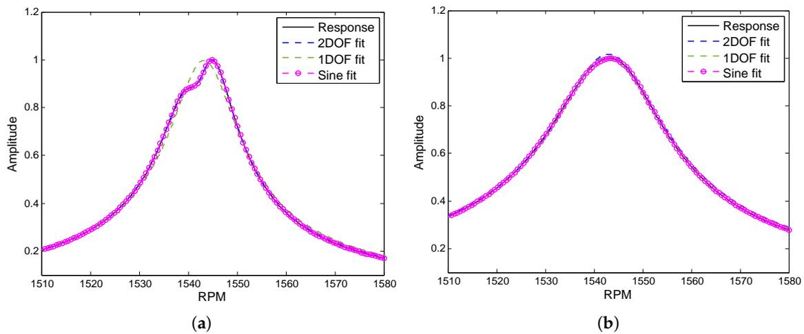
**Figure 12.** Comparison of non-dimensional amplitudes obtained by different fitting methods for SD = 0.10, (a) EO = 10,  $\zeta_{1,2} = 0.003$ , (b) EO = 10,  $\zeta_{1,2} = 0.006$ .
