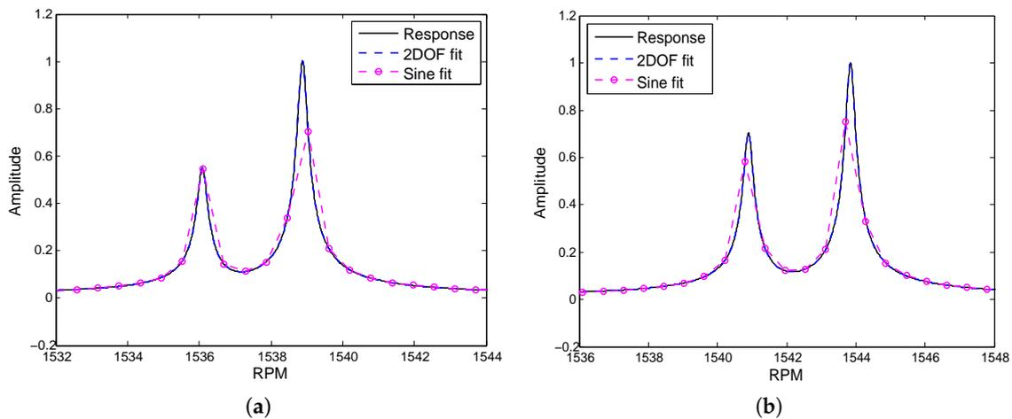
**Figure 10.** Comparison of non-dimensional amplitudes obtained by different fitting methods for  $EO = 10$  and  $\zeta_{1,2} = 0.0001$ , (a)  $SD = 0.05$ , (b)  $SD = 0.10$ .
