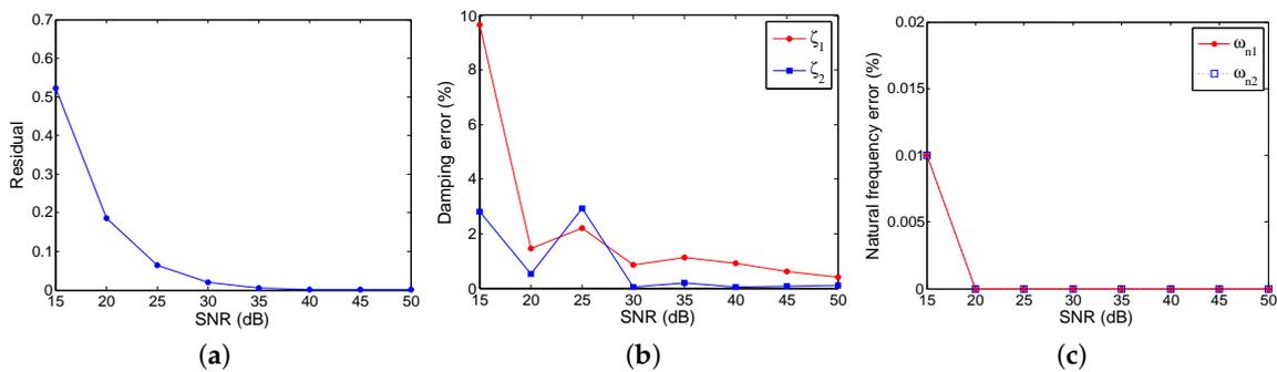
**Figure 14.** Effect of noise on the fitting residual, damping ratio and natural frequency for  $EO = 5$ ,  $\zeta_{1,2} = 0.002$  and  $SD = 0.10$ , (a) fitting residual, (b) error in damping ratio, (c) error in natural frequency.
