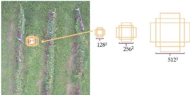
Figure 3. Example of anchors on real case images on the left. On the right, anchor scales ( $128^2$ ,  $256^2$ ,  $512^2$ ) and aspect ratios (1:1- squared shape, 1:2- horizontal rectangular shape and 2:1- vertical rectangular shape) for the PASCAL challenge.
