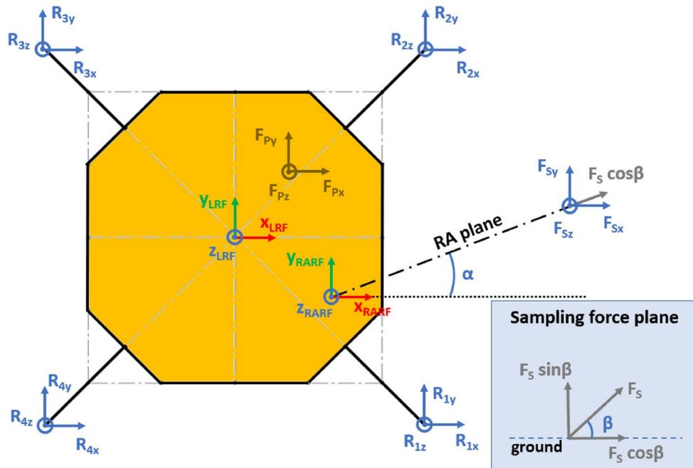
**Fig. 7** Main geometric parameters (XY plane view) for the 4-legged lander. Qualitative scheme, not to scale
