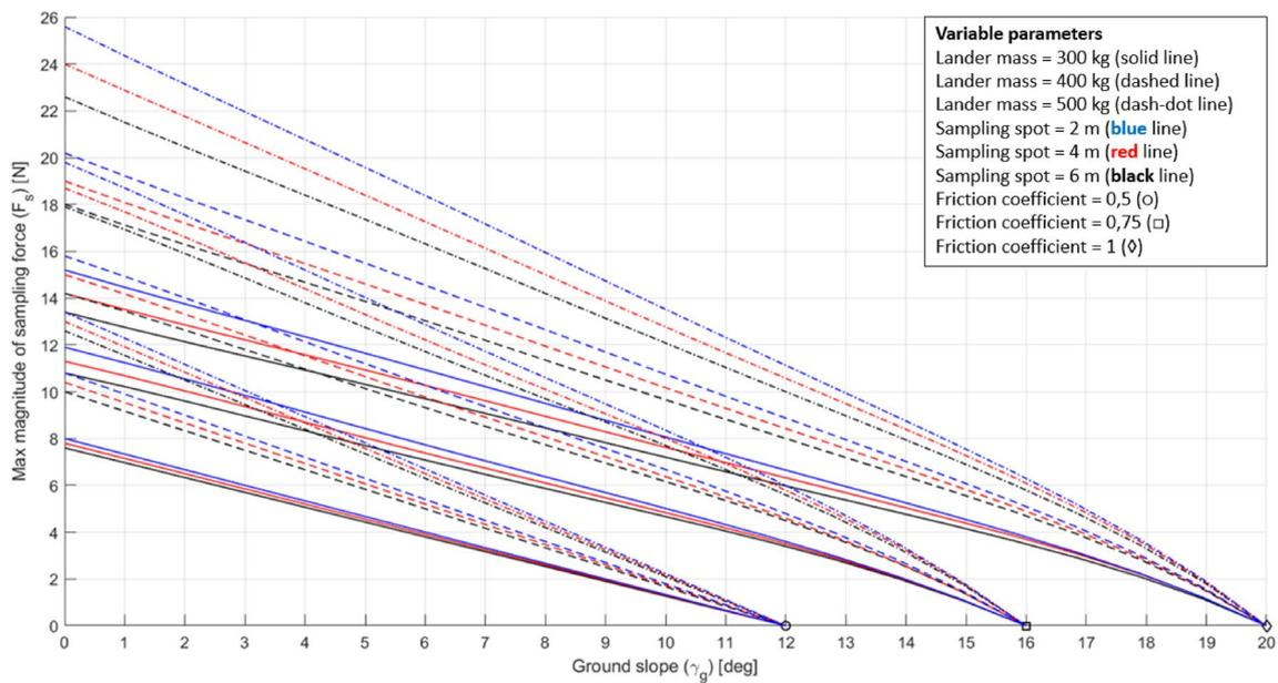
**Fig. 22** DE of the 4-legged lander for the Enceladus lander case study. The ground slope is reported in absolute value for convenience
