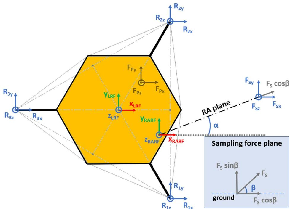
**Fig. 3** Main geometric parameters ( $XY$  plane view) for the 3-legged lander. Qualitative scheme, not to scale
