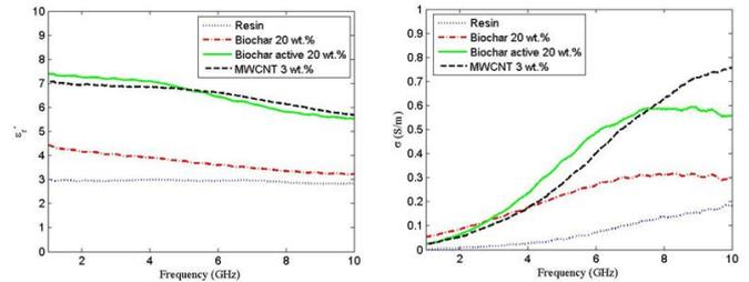
Fig. 2. Real permittivity (left panel) and conductivity (right panel) of Biochar as is, activated (both at 20 wt.%), MWCNTs (3 wt.%) and Epoxy resin.
