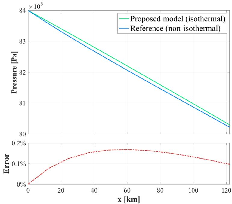
**Fig. 4** Comparison of this work's model with the non-isothermal model by Pellegrino et al. [7].
