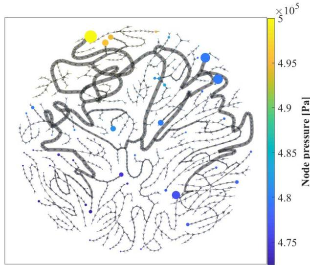
**Fig. 3** Visualization of results of the test simulation carried out on Network 1. The size of the network nodes varies with the gas flow rate consumed (or injected) by the node. The thickness of the edges increases with the quantity of gas flowing in the corresponding pipelines. Arrows indicate the direction of the flow in each edge.
