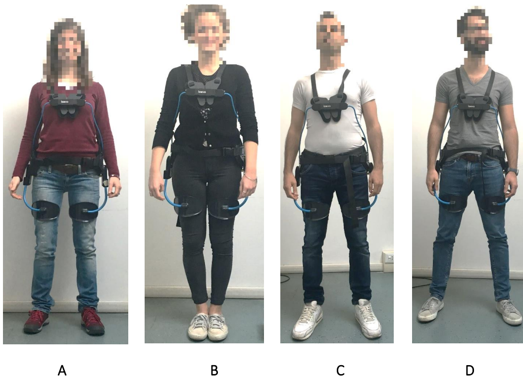
Figure 4.1.6: Front view of four subjects with different height, anthropometry and gender wearing passive Laevo exoskeleton.
