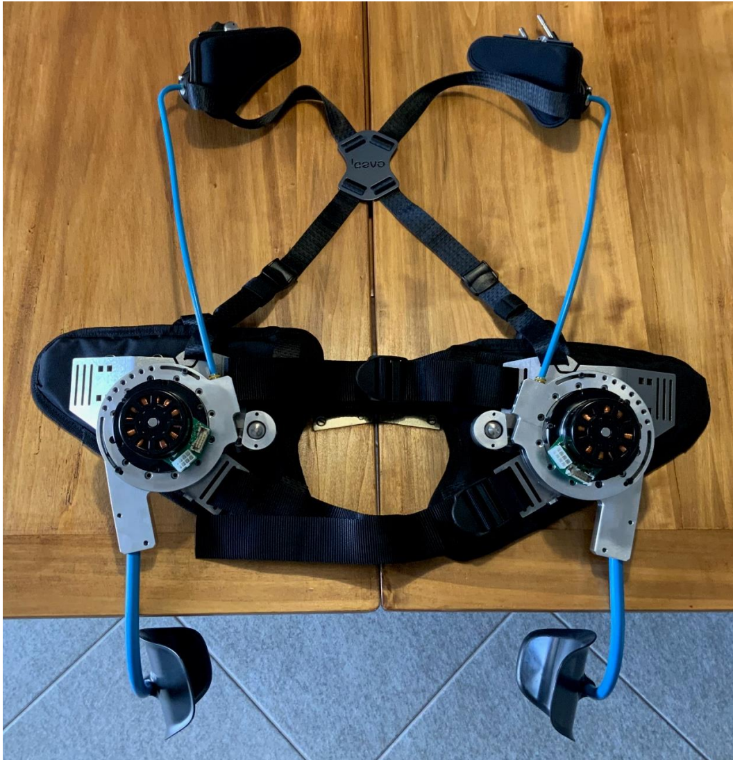
Figure 8.6.6: Final assembly of the powered exoskeleton.
