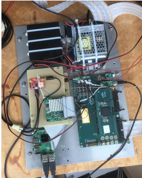
**Figure 2.** Photo of the electronics of one of the POLA detectors, before enclosing it in its aluminum box. Connections to the sensors used can be seen.
