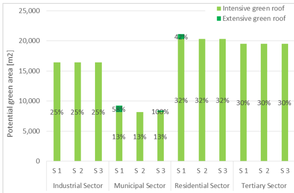
Figure 11. Scenarios 1-2-3: Analysis results of the potential intensive (flat roof) and extensive (pitched roof) green roofs
