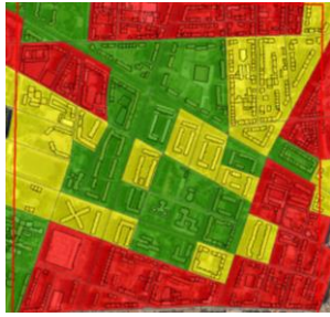
Figure 10. Scenario 3: Building block classification according to three classes of thermal comfort conditions (green: Good, yellow: Acceptable, red: Bad)
