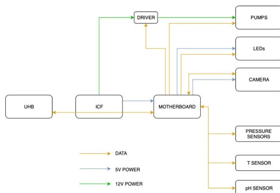
Fig.8. Electronics diagram
