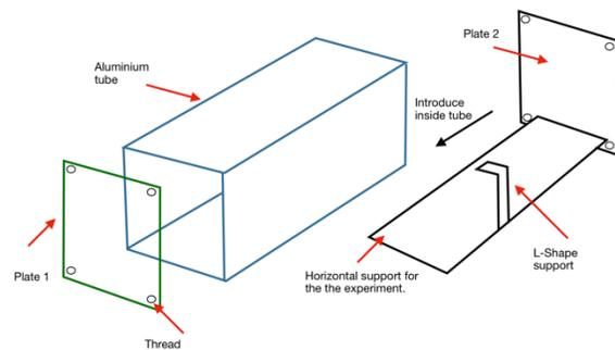
Fig. 5. Illustration of external structure assembly method
