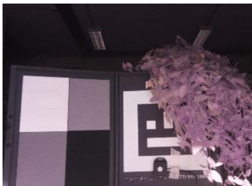
Figure 4. Picture of the calibration scene taken by the NoIR camera. On the left the calibration target composed by four panels (white, light grey, dark grey and black). On the right, side on the picture a plant. At the bottom of the picture is visible the irradiance sensor of the hyperspectral.
